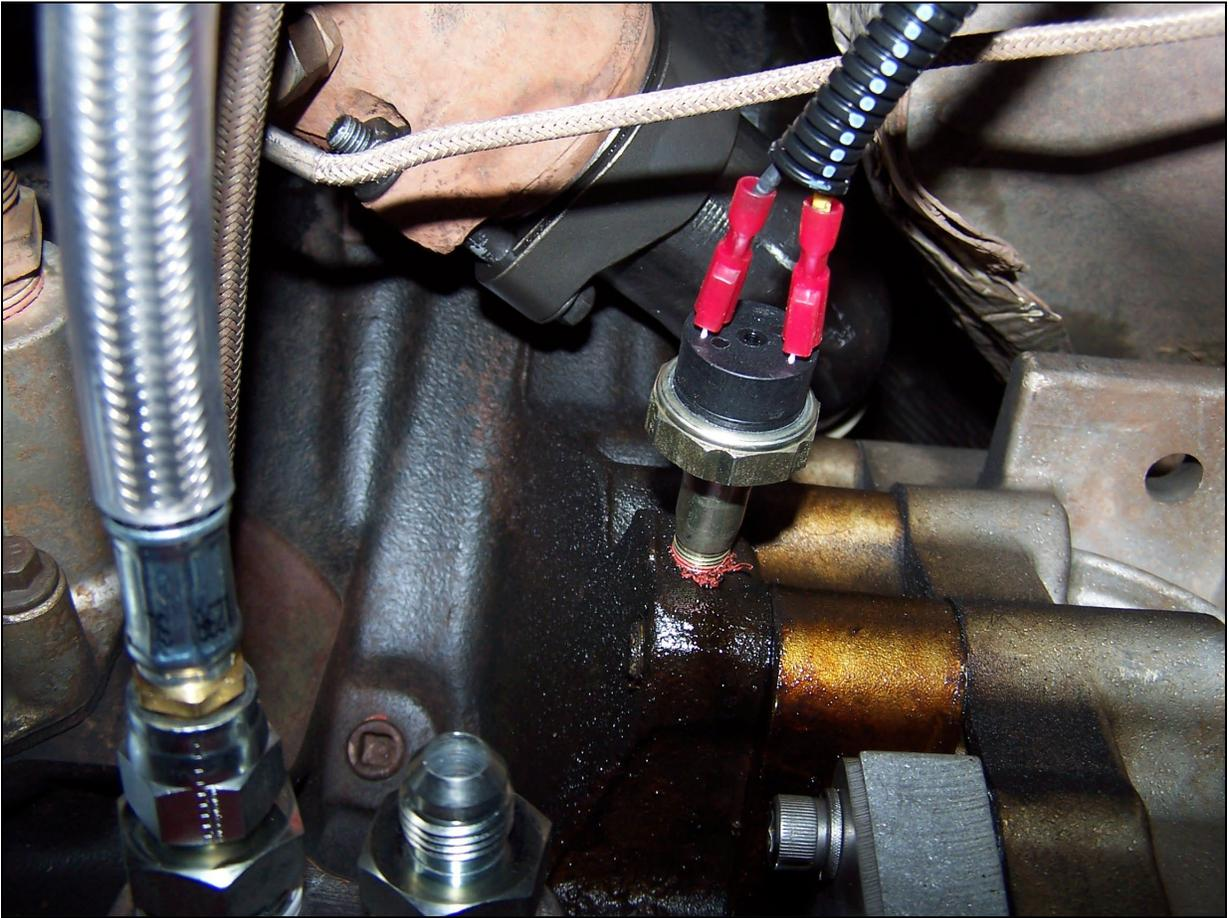
FIGURE 9 – OIL PRESSURE SWITCH INSTALLED – DRIVERS SIDE OF ENGINE BEHIND OIL FILTER
