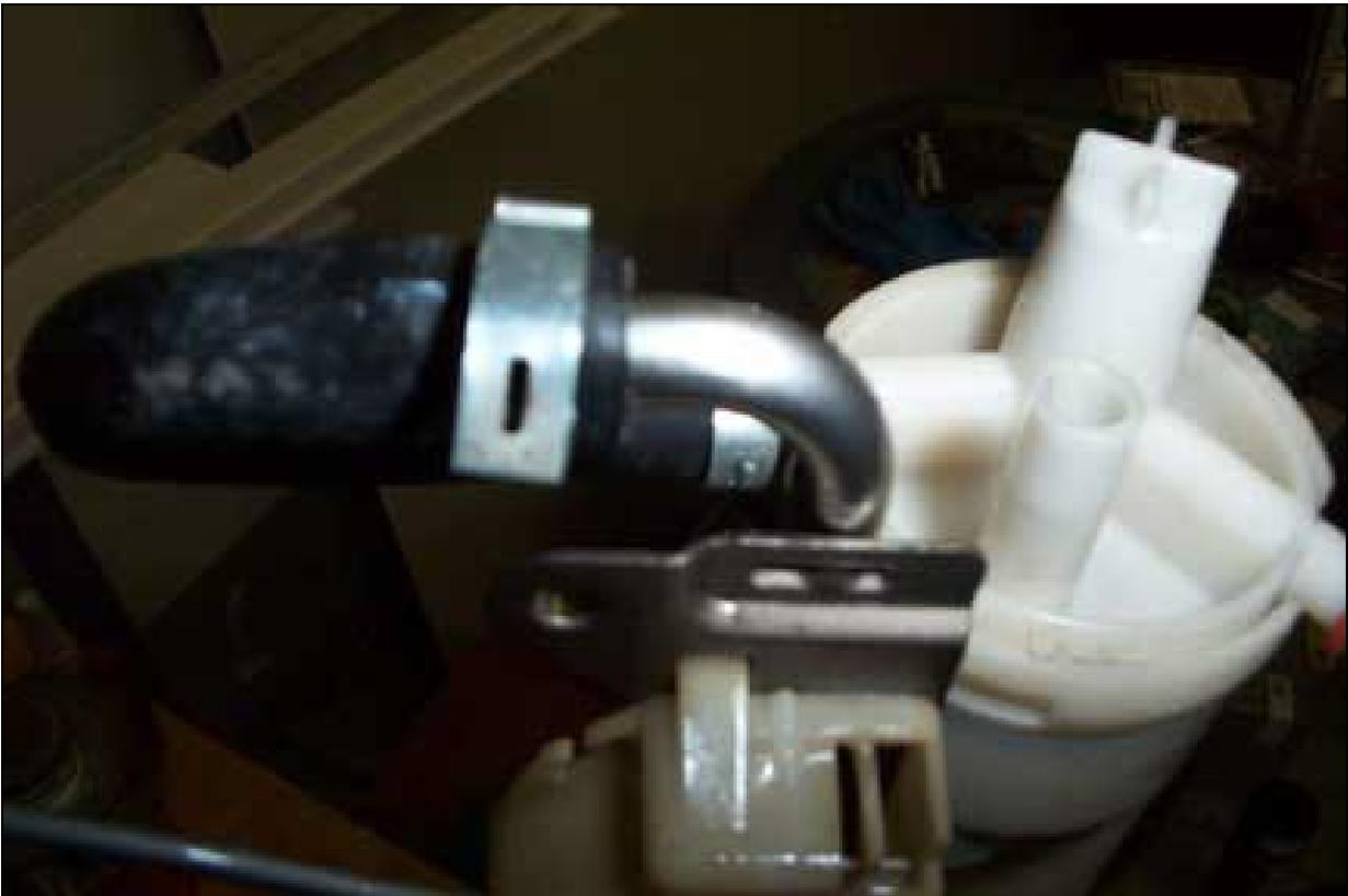
Figure 4 - Cutting The Factory Return Line Hose Clamp
