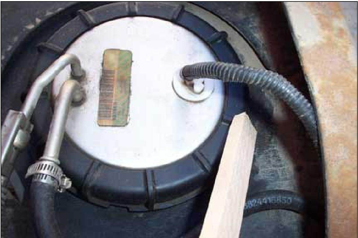
Figure 2 - Removing The Sending Unit Retention Ring
