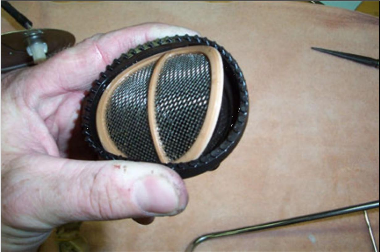
Figure 7 – Removing Filter Screen From Strainer
