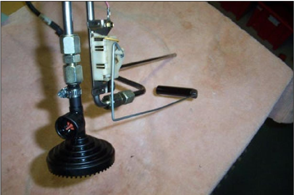
Figure 10 – Sending Unit Assembly Ready for installation
