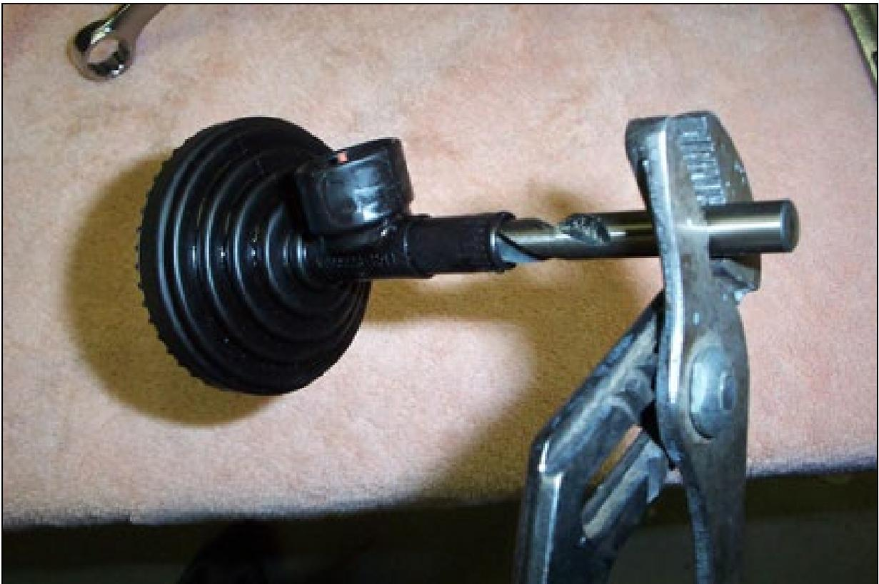
Figure 8 – Clearancing Pickup Strainer for Pickup Tube
