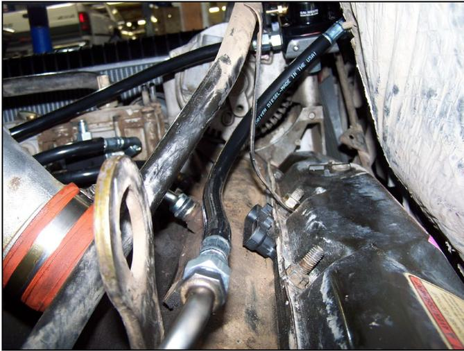
FIG 31 : Passenger Side Return Hose Installed
