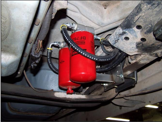
FIG 37 : Driven Diesel Pre/Post Fuel Filter Kit
