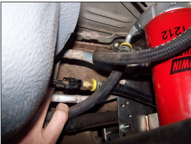
FIG 35 : Return Adapter and Return Hose Location
