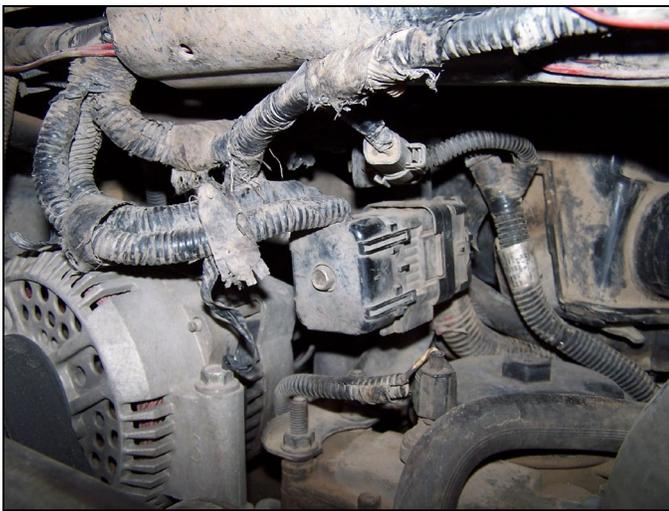
FIG 3 : Main Engine Harness Connector
