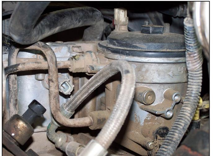
FIG 18 : Fuel Filter Canister (from rear)
