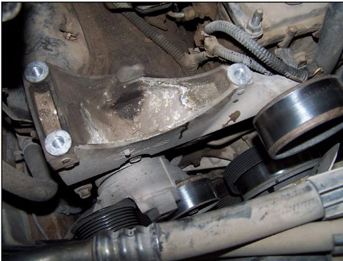
FIG 9 : Belt Tensioner – Lower Center of Photo
