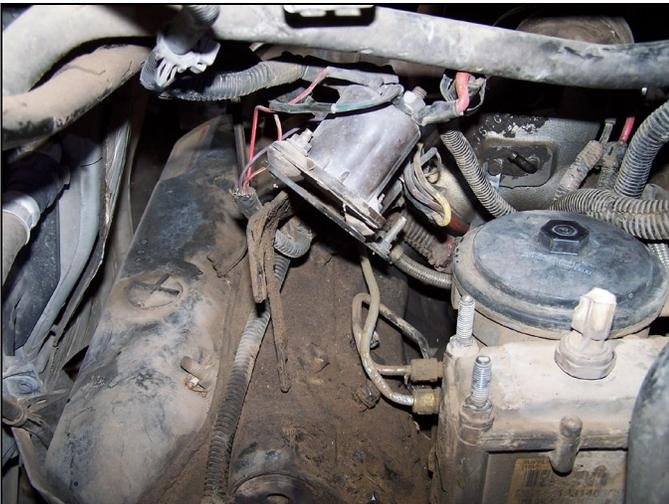
FIG 17 : GP Bracket Moved – Fuel Lines Exposed
