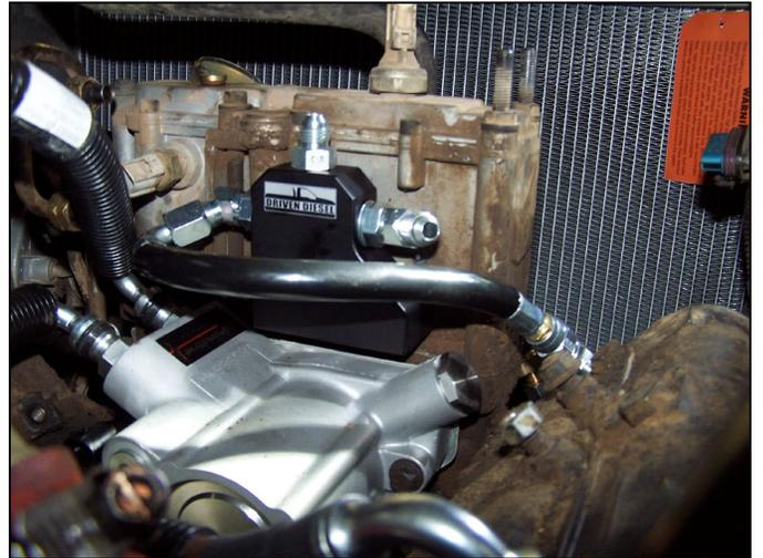
FIG 26 : Fuel Bowl Delete Block Installed
