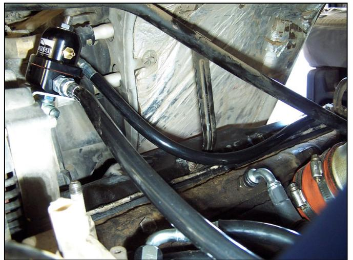
FIG 34 : Driver and Passenger Hoses Connected to Reg
