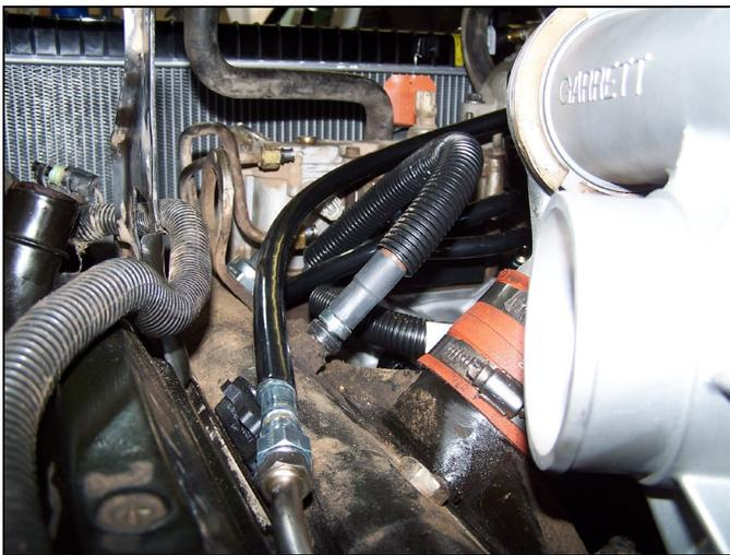
FIG 33 : Driver Side Return Hose Installed
