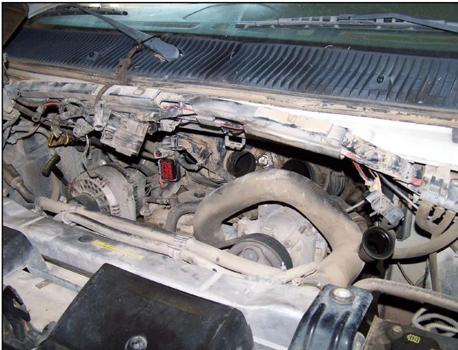
FIG 5 : Cowl Harness Pulled Up Out of Way
