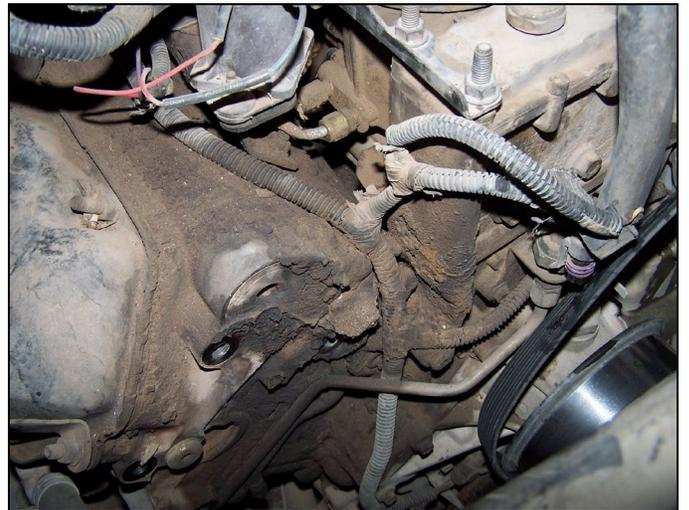
FIG 10 : Alternator Bracket Removed
