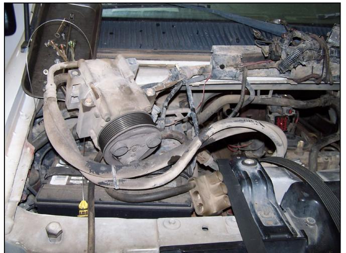
FIG 12 : A/C Compressor Moved Off Engine
