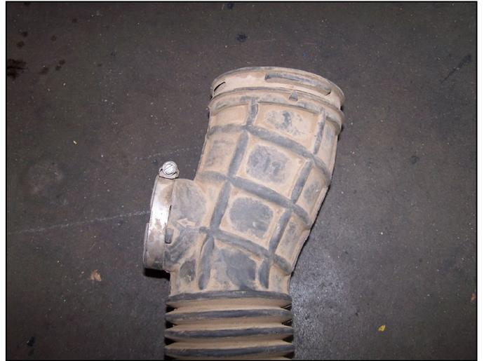
FIG 2 : Intake Hose – Showing Resonator Box Clamp
