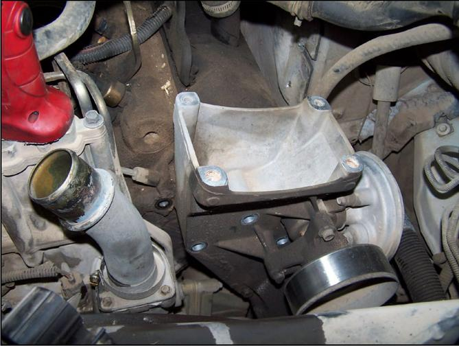
FIG 13 : A/C Compressor Bracket
