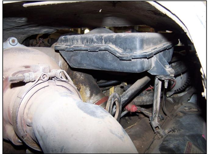
FIG 8 : Air Intake Resonator Box
