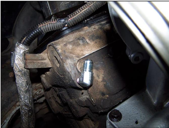
FIG 21 : Driver Side Rear Fitting Installed
