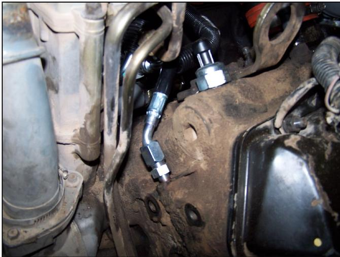
FIG 27 : Drivers Front Feed Line Connected
