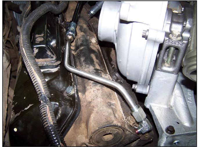
FIG 32 : Driver Side Return Tube Installed
